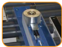
Self-tensioning & tracking side drives simplify belt replacement
